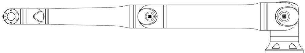
4. Verify the robot arm can maintain the position without support and without activating Freedrive.
