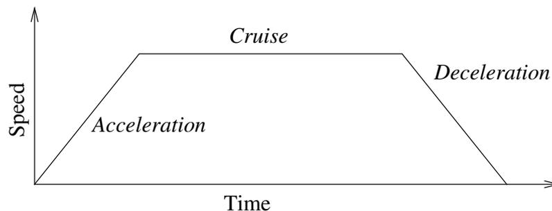
**31.1:** *Speed profile for a motion. The curve is divided into three segments: acceleration, cruise and deceleration. The level of the cruise phase is given by the speed setting of the motion, while the steepness of the acceleration and deceleration phases is given by the acceleration parameter.*
