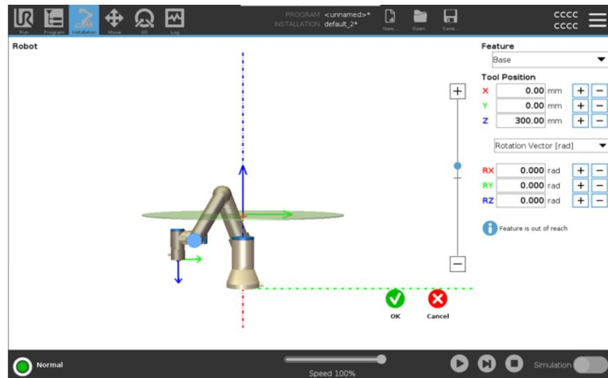
If needed it is possible to offset the plane in either positive or negative Z-direction later in the safety settings.
