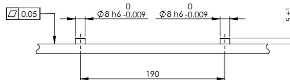
*Holes for mounting the robot, and where to drill holes and mount the screws.*
