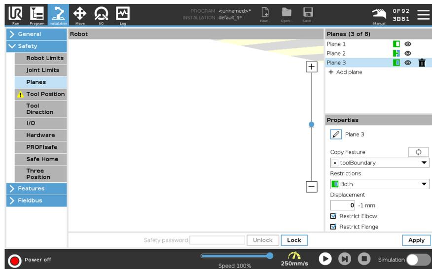
**Elbow Restriction** You can enable **Restrict Elbow** to prevent robot elbow joint from passing through any of your defined planes. Disable Restrict Elbow for elbow to pass through planes. The diameter of the ball that restricts the elbow is different for each size of robot.
