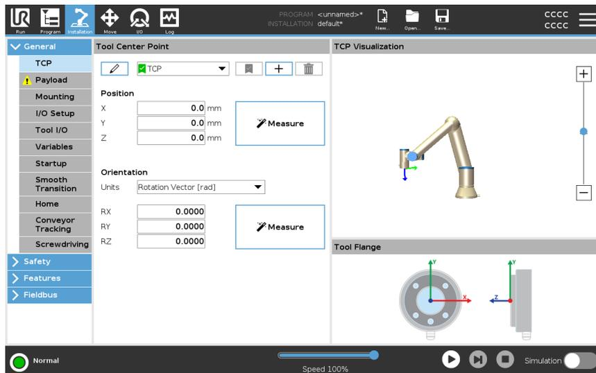
**Position** The X, Y, Z coordinates specify the TCP position. When all values (including orientation) are zero, the TCP coincides with the center point of the tool output flange and adopts the coordinate system depicted on the screen.
