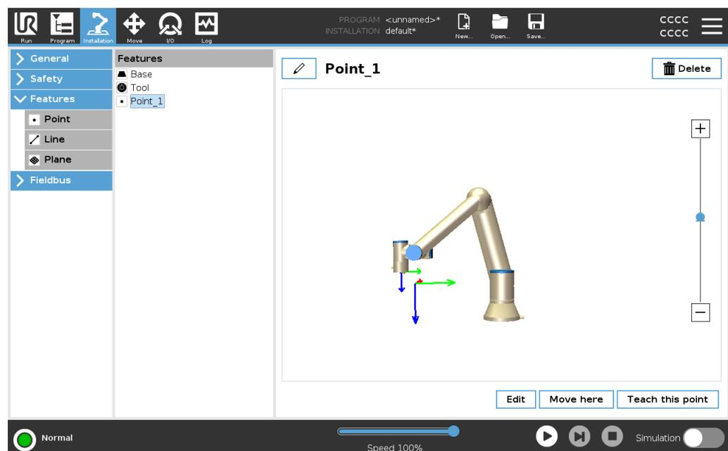
**Line feature** The line feature defines lines that the robot needs to follow. (e.g., when using conveyor tracking). A line  $l$  is defined as an axis between two point features  $p1$  and  $p2$  as shown in figure 24.13.
