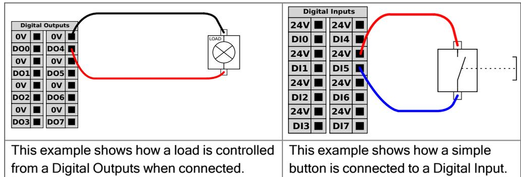
**Communication with other machines or PLCs** You can use the digital I/O to communicate with other equipment if a common GND (0V) is established and if the machine uses PNP technology, see below.
