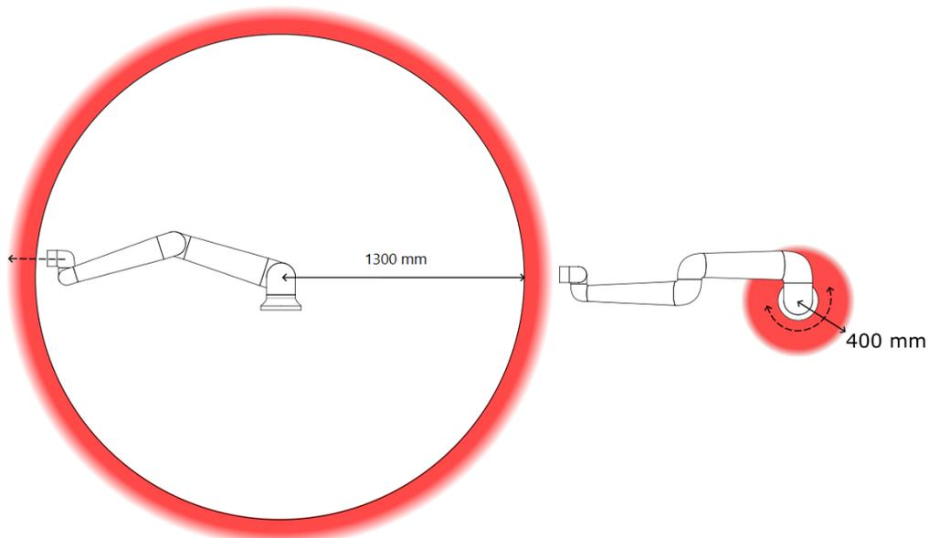
**3.1:** *Due to the physical properties of the robot arm, certain workspace areas require attention regarding pinching hazards. One area (left) is defined for radial motions when the wrist 1 joint is at least 450 mm from the base of the robot. The other area (right) is within 200 mm of the base of the robot, when moving tangentially.*
