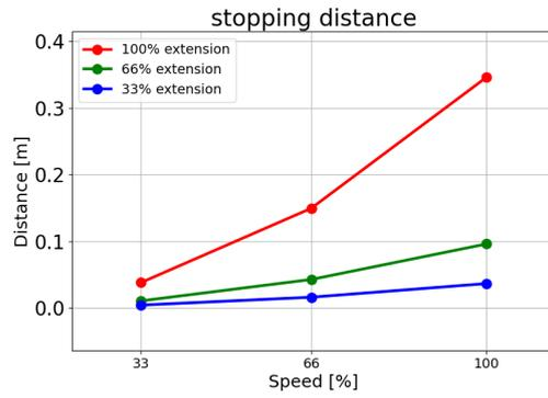
Stopping distance in meters for 66% of 30 kg
