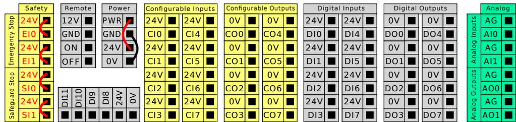
You can use the horizontal Digital Inputs block (DI8-DI11), illustrated below, for quadrature encoding Conveyor Tracking (see [Common specifications for all digital I/O on the next page](#)) for these types of input.
