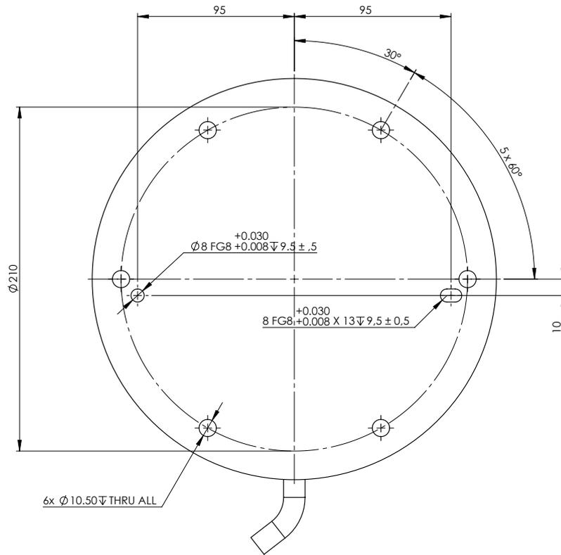
**Mounting Plate with Pins for Robot Base**
