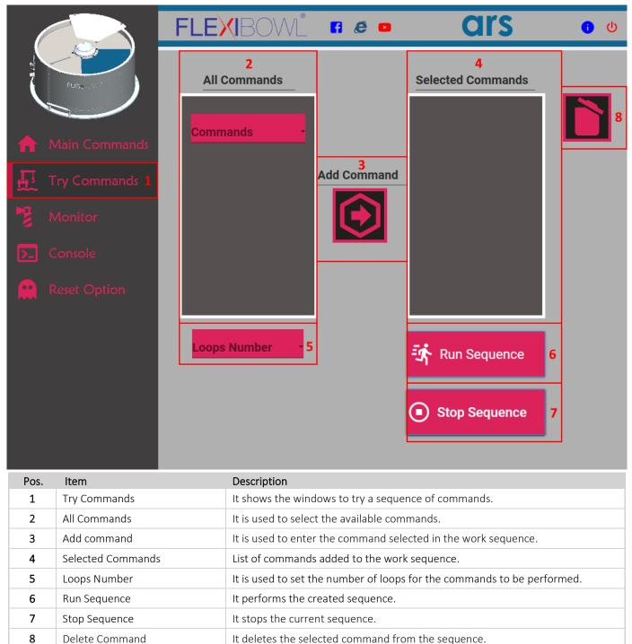
**Note:** To use the parameters set in the previous command windows, you must first save them inside the Flexibowl<sup>®</sup>. This can be done in the Option window by pressing the Send Parameters to Flexibowl<sup>®</sup> button.
