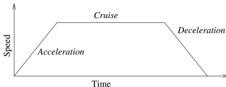
**30.1:** Speed profile for a motion. The curve is divided into three segments: acceleration, cruise and deceleration. The level of the cruise phase is given by the speed setting of the motion, while the steepness of the acceleration and deceleration phases is given by the acceleration parameter.
