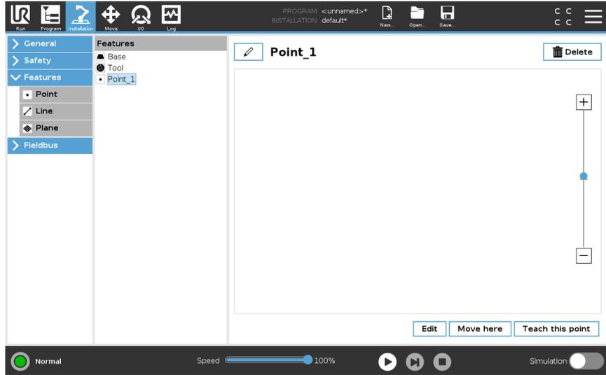
Use Edit to place and move features without moving the robot arm, so the feature can be placed outside of the robot arm's reach.
