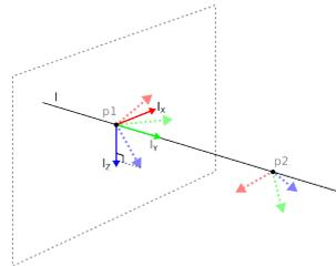
Here you can see the axis directed from the first point towards the second point, constitutes the y-axis of the line coordinate system. The z-axis is defined by the projection of the z-axis of  $p1$  onto the plane perpendicular to the line. The position of the line coordinate system is the same as the position of  $p1$ .
