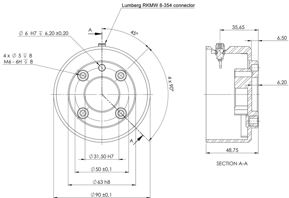
Dimensions and hole pattern of the tool. All measurements are in millimeters.
