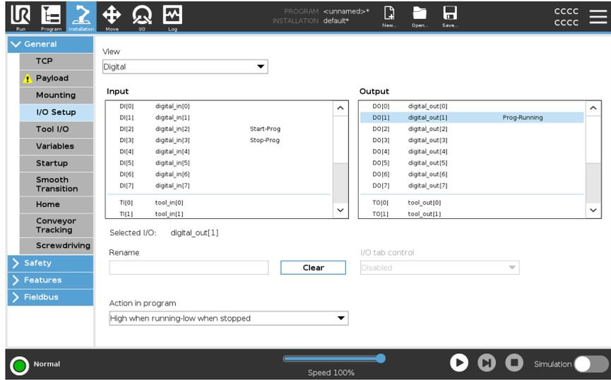
**I/O Signal Type** To limit the number of signals listed under **Input** and **Output**, use the **View** drop-down menu to change the displayed content based on signal type.
